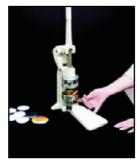
**Step 6 -** Using the ejector pin on the right hand side of the bottom die, push up to eject the completed badge.
