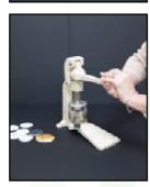
**Step 3 -** Pull the handle down until the top die engages with the bottom die. Gently release the handle to the upright position and you will notice that everything but the badge back has transferred to the top die. This is normal.
